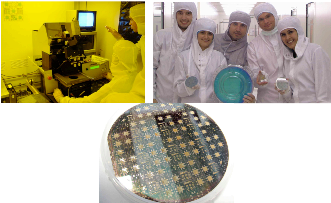
Figure 1. ESONN students operating double side photolithography and in clean room (top pictures). Realized MEMS and MOS devices on 4" wafer (bottom picture).
