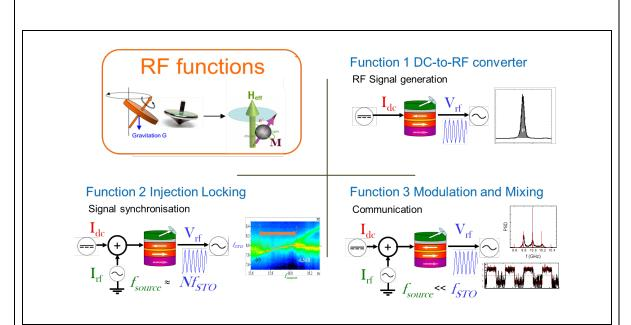
**Figure 1**: Top left: Equivalence of a spinning top and the magnetization dynamics; Top right: RF-DC conversion: injection of a DC spin polarized current results in an rf voltage signal due to steady state excitations. Bottom: By adding an additional RF current one can (left) injection lock the device ( $f_{\text{source}} \approx f_{\text{STO}}$ ) or (right) frequency modulate the output signal ( $f_{\text{source}} < f_{\text{STO}}$ ).
