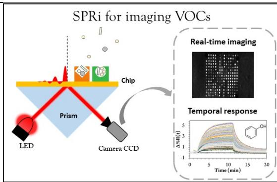
**Figure 1:** Schematic illustration of the electronic nose composed of a microarray and an optical detection system SPRi. For each VOC, the electronic nose can generate temporal response and an image pattern, which behaves like a fingerprint suitable for differentiation and identification of the samples.
