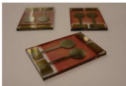
Figure 1: Standard bulk hetero-junctions solar cells made during this practical.
