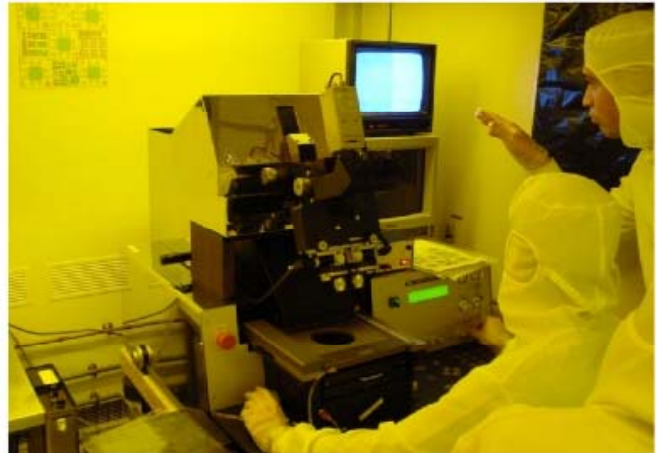
Figure 1. Left: A MEMS wafer similar to the ones that will be simulated and characterized during the practical. Right: Double-side photolithography tool in clean room.
